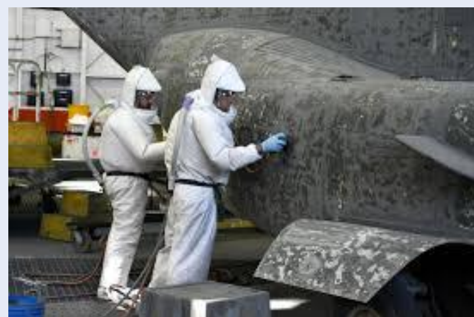
Fig. 1: Depainting by chemical stripping. Shown is the manual debris removal step via sanding 1 .
