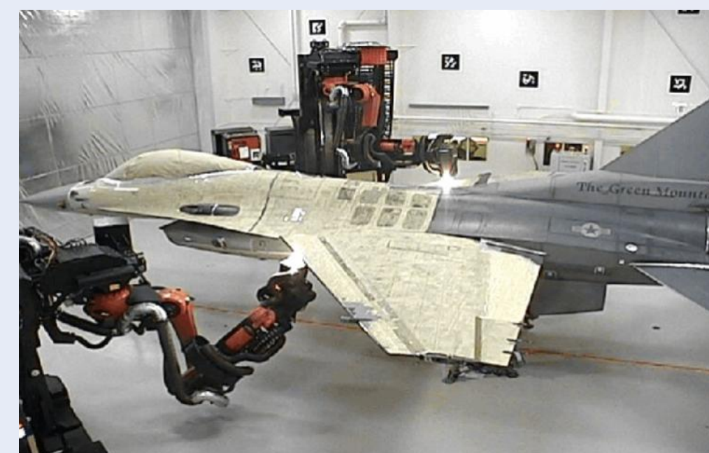
Fig. 2: Depainting by laser ablation. Shown is a Titan Robotics laser system actively ablating 2 .
